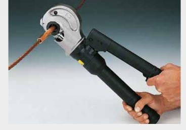
HT 120 features a double speed action: a fast advancing speed for rapid approach of the dies to the connector and a slower more powerful speed for crimping.
