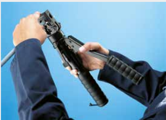
The operator can advance the dies using only one hand, leaving the other hand free to position the connector.
