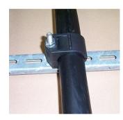
4) Important: Do not over tighten the clamp. The clamp should secure the cable but does not need to be so tight that the cable bulges at either side of the clamp or becomes angled excessively.
