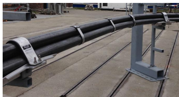
A photo of the short circuit test rig for Centaur Trefoil. Testing was carried out at ZKU Laboratories in Prague, CZ.
