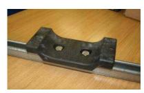
Fix the bottom half of the cleat to the support structure using M10 or M12 fixings as appropriate.
