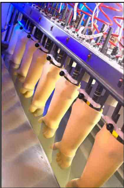
Testing gloves to the EN60903 & IEC60903 Standard
