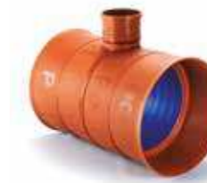
Ridgisewer 90° unequal junctions 110 & 160mm branches are for EN1401 pipes. 150mm branches are for Polysewer. Order seals separately if required.
