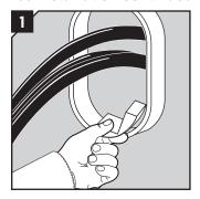
Insert the lubricated RM 60/0 RC modules in the bottom corners.
