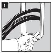
Insert the lubricated RM 20/0 RC modules in the bottom corners.
