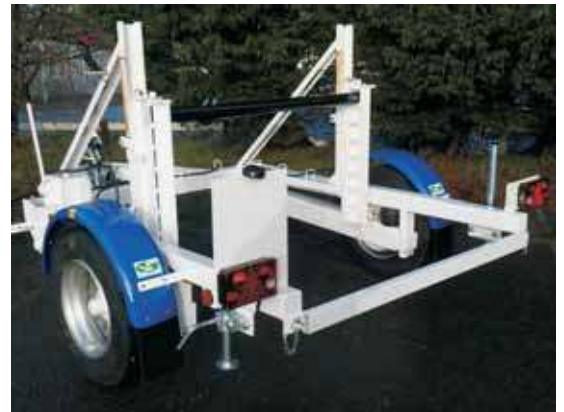
Rear of CD60 Cable Drum Trailer
