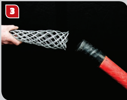
3 The grip should then be placed over the end of the conductor...
