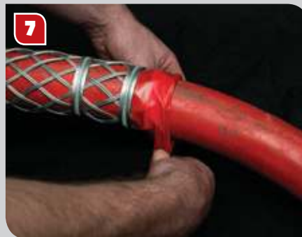
7 Tape should then be wound around the end of the cable grip furthest away from the eye ends.
