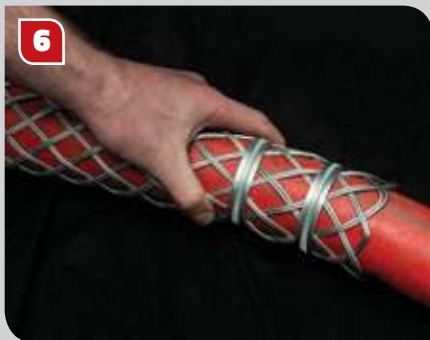
6 Once the cable grip is in place on the conductor, two clamps should be fitted to the end of the grip (as shown). We recommend between 1 ¼" (30mm) and 2 ¼" (55mm) away from the end of the cable grip.
