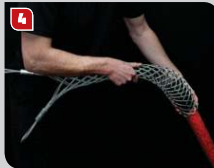
4 ...and pushed over the conductor.
