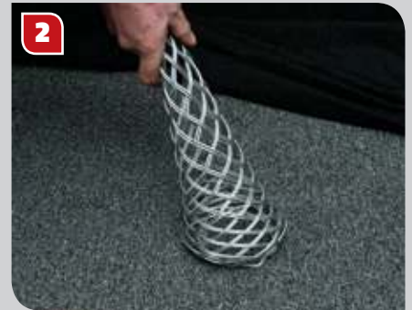
2 Prior to use, the lattice at the end of the grip needs to be widened. This can be easily achieved by pressing the end of the grip against a hard surface, which causes the lattice to expand.
