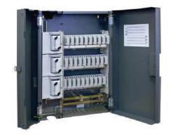
Mild steel wall mounting distribution boards for 3 phase systems configurable with either a single incoming bank of triple pole J type slotted tag fuses or with an additional outgoing bank of triple pole J type fuses for mixed developments requiring a split supply greater than 100 A.
