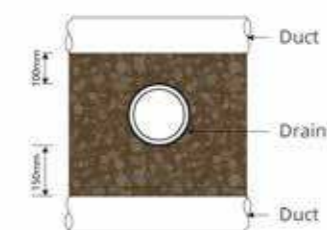
Minimum clearance between duct and drain
