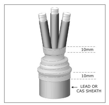
With tension, wrap the Grey Mastic Tape around the Crutch area and overlap the Stress Control Tubes and Lead or Aluminium Sheath by approx 10mm.
