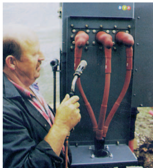
Picture shows XLPE and PILC 12kV Joints and Terminations undergoing type testing to BS 7888 and Cenelec standard HD 628 S1 and HD 629.1 S1 ASTA Test Report Available
