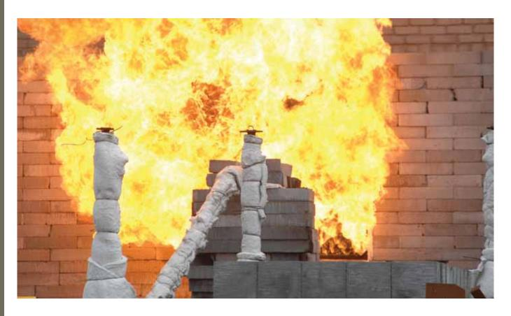
Offering 2 hour fire protection for both integrity and insulation, ACTIFOAM has been tested in accordance with the most stringent fire test procedure, BSEN1366-3 (will soon become mandatory). With the addition of a FIWA (or NOFIRNO) layer, the system also becomes gastight and watertight.
