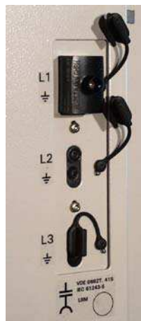
Fig. 13: LRM plug-in sockets
