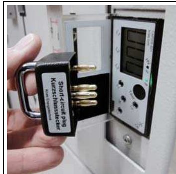
Fig. 116: Short-circuit plug, make Kries, order number 2500029
