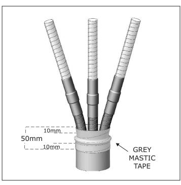
Clean the Metal Sheath. With tension, wrap the Grey Mastic Tape around the Cable Crutch area and extend onto the Metalised Screen Papers and Metal Sheath by a minimum of 10mm
