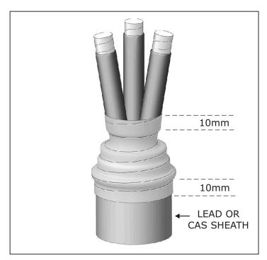
With tension, wrap the Grey Mastic Tape around the Crutch area and overlap the Stress Control Tubes and Lead or Aluminium Sheath by approx 10mm.
