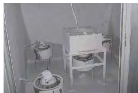
Test object in the dust test chamber after the dust test.
