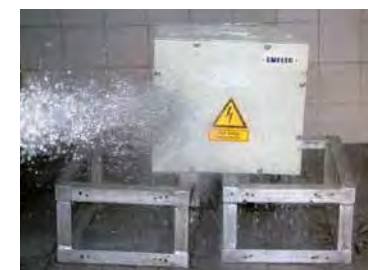
Test object during the test water jet onto front side
