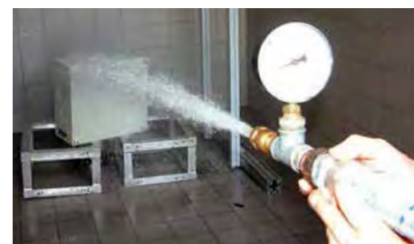
Test object during the test water jet onto rear side
