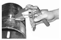
2. With ratcheting action, tension the band until clamp is tight. If necessary, band may be repositioned by releasing tension with levers.
