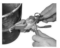
2. With ratcheting action, tension the band until clamp is tight.
