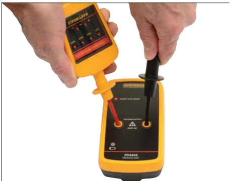
PD440S for proving 440V indicators
