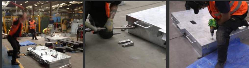
The Citadel range has been extensively tested by BRE to ensure it meets the demands of Level 4 of LPS 1175: Issue 7.
