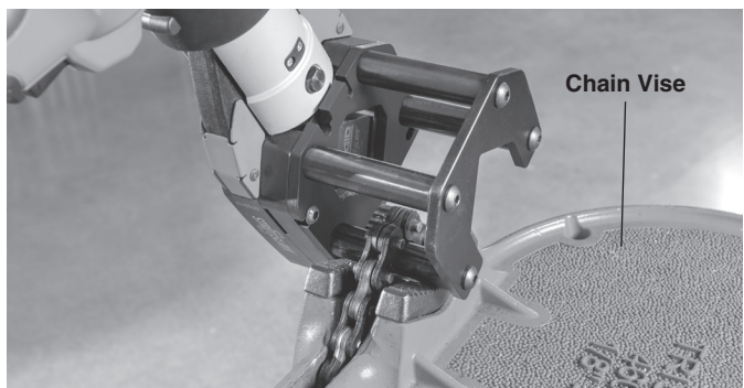
Figure 5 – Strut Shear Head Mounted in Chain Vise
