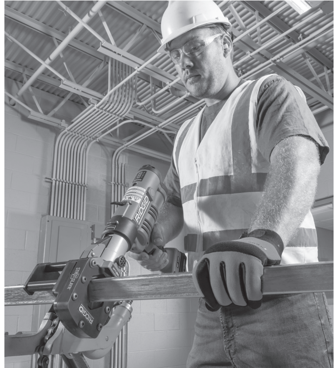
Figure 8 – Shear In Use
