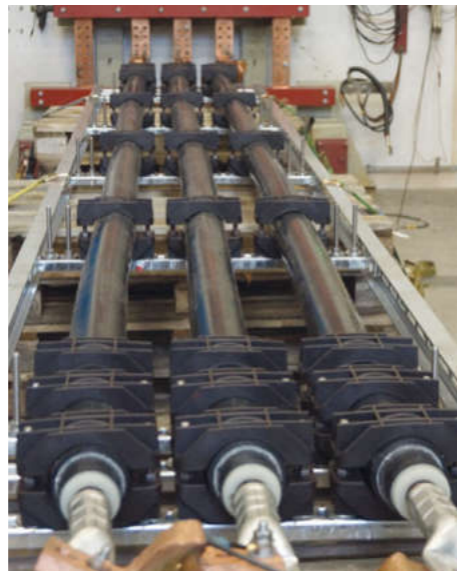
After the first short-circuit, with no damage to the cables or clamps, a second test is performed on the same arrangement with the same peak short-circuit current.
