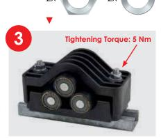
Tighten nuts with an appropriate torque wrench alternately only up to the specified tightening torque. Do not use self-securing/ self-locking nuts, this prohibits a defined tightening torque.
