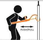
Capture and control suspended tubulars or cylindrical objects 3"-10" in diameter
