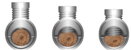
Spring assisted terminal: Stainless steel ring
